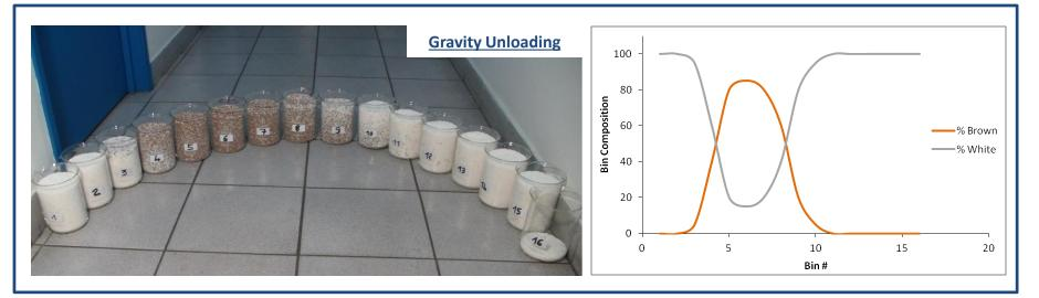
After Gravity dump, SAS can trace back the position of the catalyst in the reactor.
